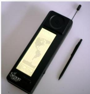
world's first so-called "smart phone". It only had two buttons: on/off and volume. Access to all other capabilities was via a resistive film touch sensor that covered the display that made up the entire front of the device. This gave access to the phone, note pad (on which one could enter text with a graphical keyboard or be hand-drawn with the stylus), address book, email, fax, calendar, games, etc. Functions are accessed by touching the
