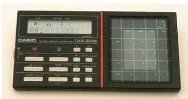
the year it was released. It was remarkable in that one could enter data either by using the mechanical keypad, or by printing the characters, one on top of the other, on the touch pad on the right. In this latter regard, it used the same basic technology as its sibling, the Casio AT-550 Calculator Watch, which is also in my collection.
